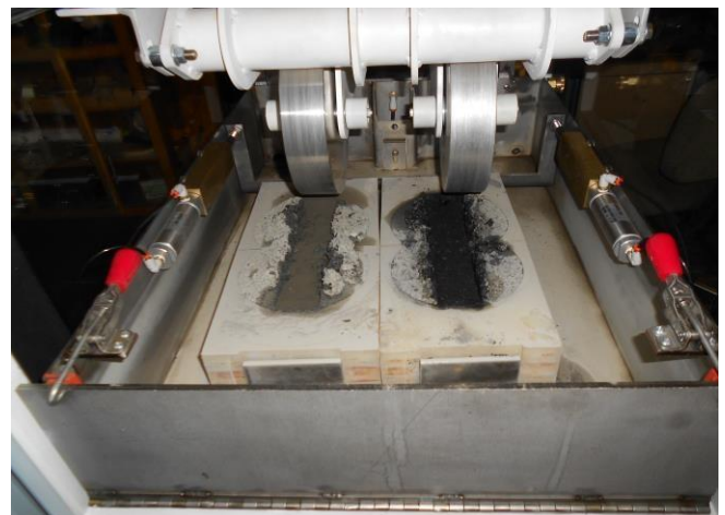
Completed Hamburg Test with Gyratory Samples
