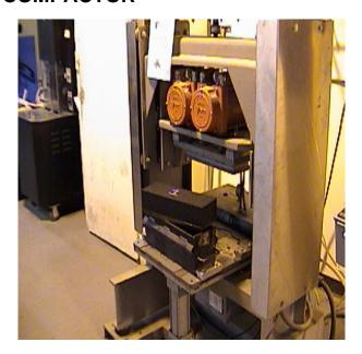
The Asphalt Vibratory Compactor (AVC) is designed to form rectangular and cylindrical test specimens used for evaluating the susceptibility of permanent deformation (rutting), fatigue cracking, and moisture damage of asphalt mixes. The AVC compacts specimens at the same amplitude, same frequency, and same relative weight that a contractor experiences with a vibratory compactor on the
