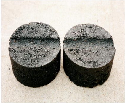
Rutted Superpave Asphalt Samples Utilizing the APA Test Method (AASHTO T340-10)
