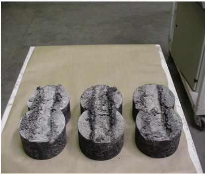
Rutted Superpave Asphalt Samples Utilizing the Hamburg Test Method AASHTO T324-22)
