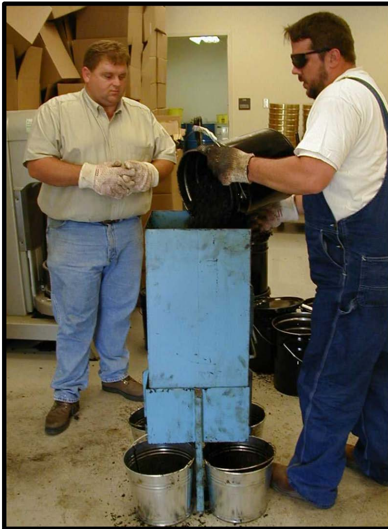
Figure 3 – Mechanical Splitter Used to Minimize Heat Loss
