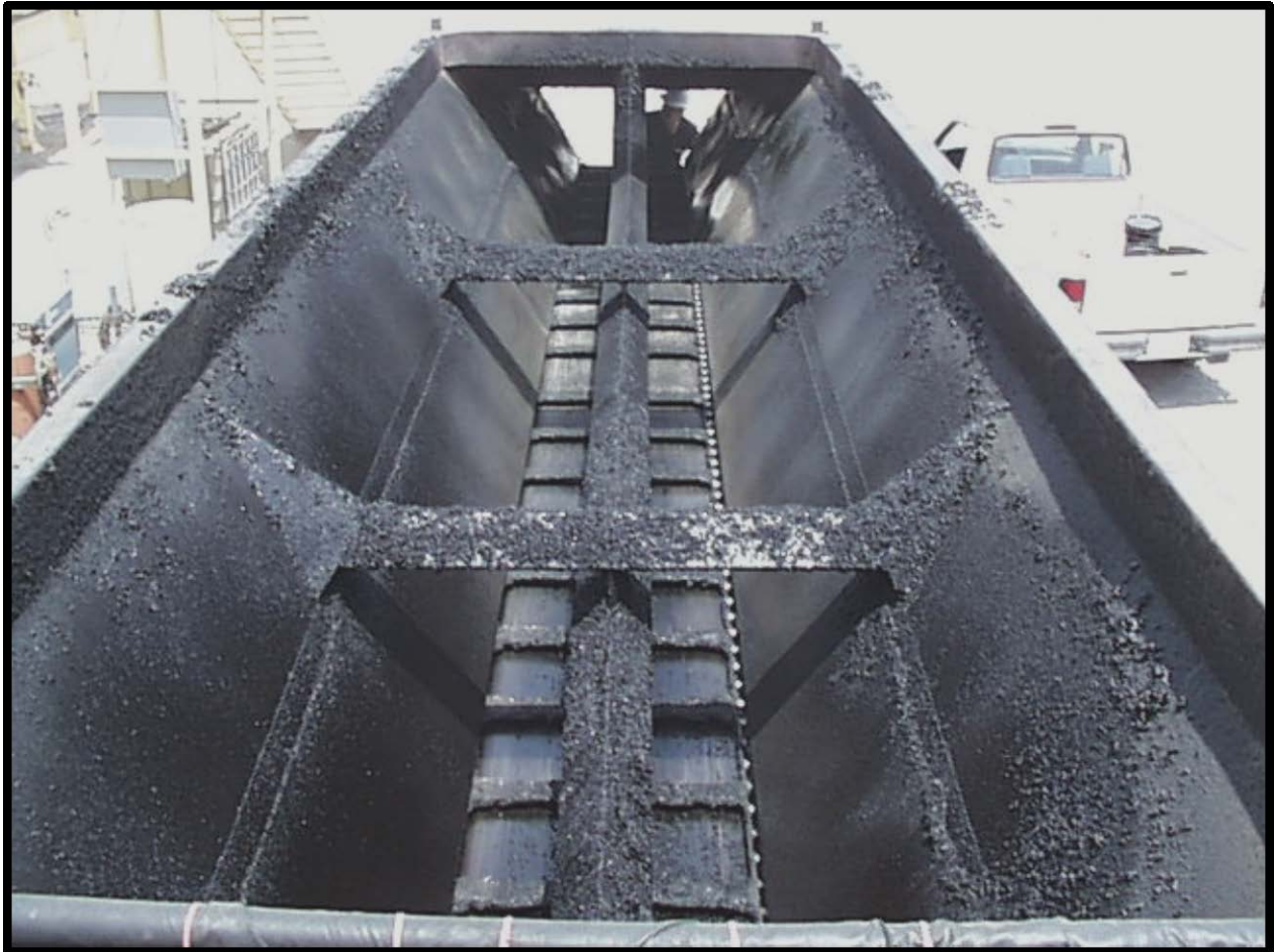
Figure 9 – Potentially Problematic Components in Flow-Boy Truck Bed
