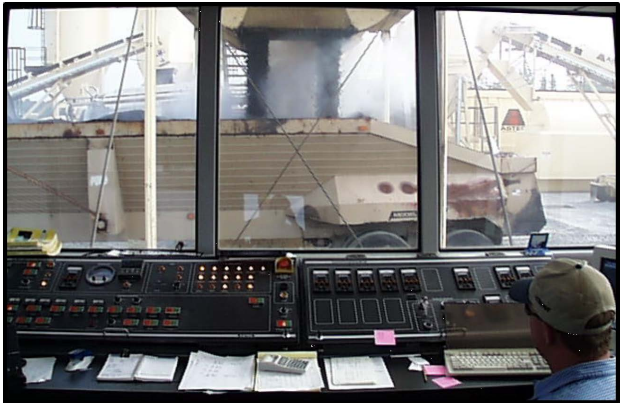
Figure 4 – Multi-Drop Flow-Boy Truck Loading Procedure to Minimize Within-Load Segregation
