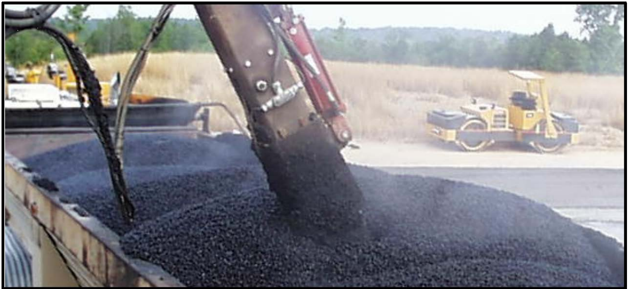
Figure 10 – Robotic Sample Head Penetrating Load Dump
