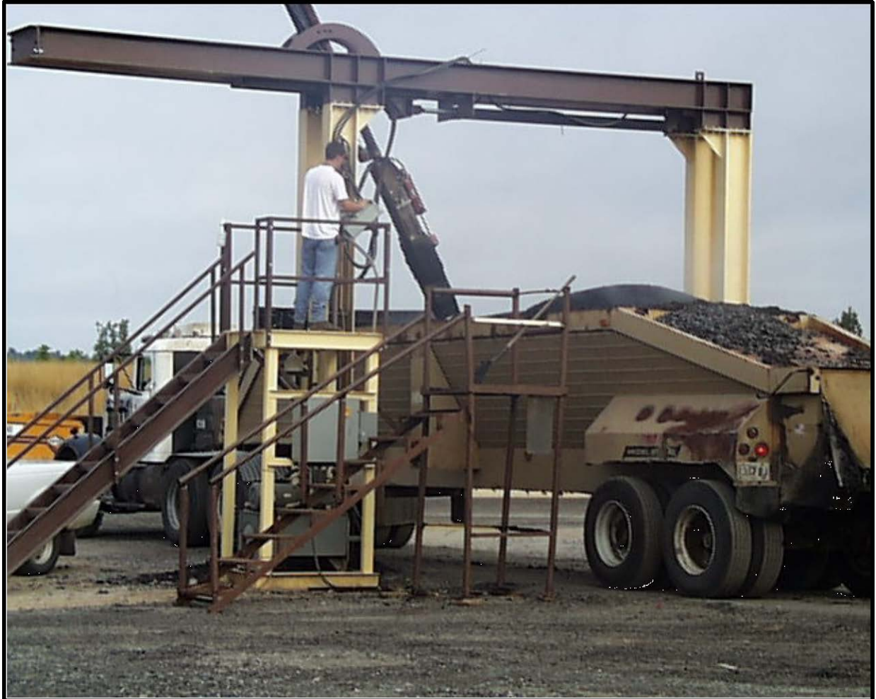
Figure 7 – Removing a Robotic Sample from Flow-Boy Truck at Plant
