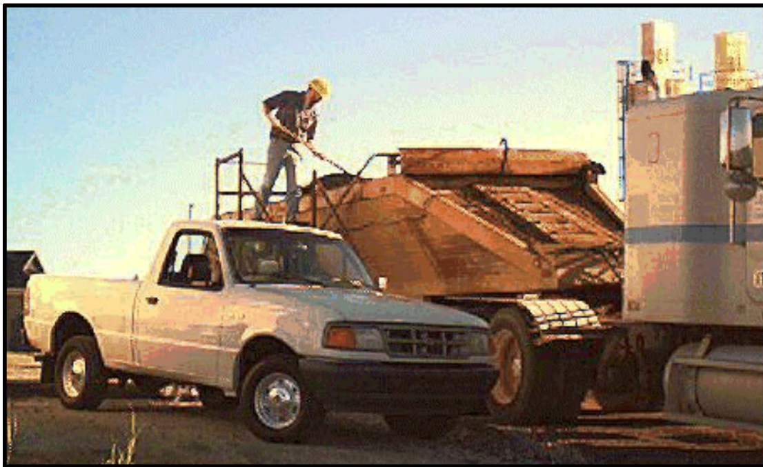
Figure 5 – Removing a Shovel Sample from Flow-Boy Truck at Plant
