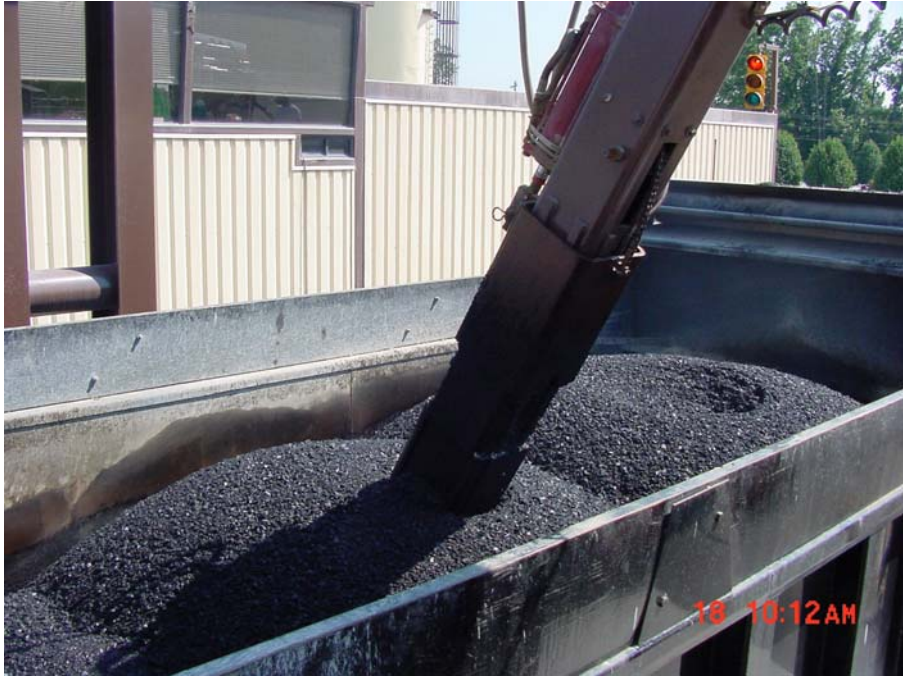
Typical of Mechanical Sampling
